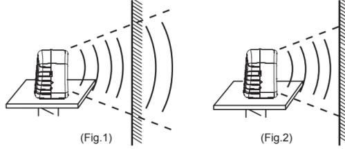
Put the main unit on the table of private area or on the surface of any objects, fix the main unit position with its detecting side (side with battery cover) facing the burglarproof direction to be detected. Within detected side's angle range  $\leq 150^\circ$ , try to avoid :
