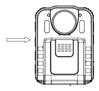
To charge the battery connect the camera to your PC using the provided USB cable. The battery charging status is displayed on the LCD icon when the camera is on and on the Charging Status Indicator Lights when the camera is off. While charging the LED is Red. When fully charged the LED will turn off.
